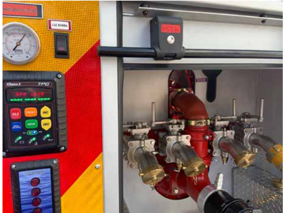
▲ Class1 instrumentation – TPG control unit and ITL40 tank level gauge.
